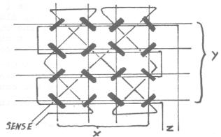
Corresponding X wires in each plane will be wired in series, as will the Y wires. One Z wire is provided for each plane and threads all of the cores in that plane - as does the sense wire. For a 4096 x 8 store we would have 64 X wires, 64 Y wires and 8 Z wires ( also 8 sense wires, but we're not concerned with these yet ). Passing the correct amount of current through one X wire and one Y wire will therefore select one core from each plane - thus selecting one word of n bits ( n planes ).
