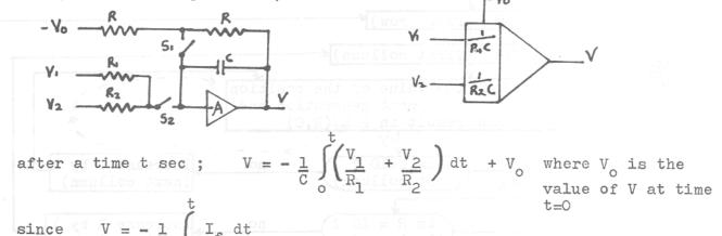
When Sl is closed and S2 open, V becomes equal to  $\rm V_{o}$  after a short time. if then Sl is opened and S2 closed, the circuit integrates the weighted sum of the input voltages according to the equation above. If s2 is then opened after a time t seconds the value of V at time t is held indefinately.
