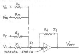
Furthermore the input of the amplifier is high impedance and may be assumed to draw no current, hence n
