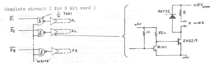
Data to be written is presented to the 7401 open collector NAND gates in inverted form -'low'to write a 'I' and 'high' to write a 'O' -on leads  $\overline{D}_1$  to  $\overline{D}_8$  ( the 's denote the inverted form ). Current will then flow in the selected Z wires when the 'write' lead is l ('high'). Other semiconductors than those shown can be used, the only critical requirements are reasonably high switching speeds (better than  $\frac{1}{4}$  uS) and sufficient current carrying capacity.
