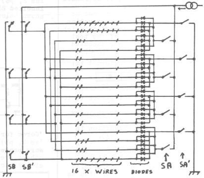
4 sets of SA switches and 4 sets of SB switches give us 4x4 = 16 combinations, thus we can uniquely select any one of the 16 wires. For a stack with 64 X wires we would need 8 sets of SA and 8 sets of SB.
