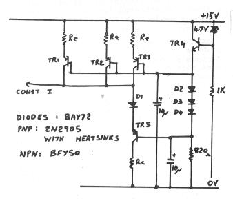
TR1,2 & 3 each supply one third of the required current, as determined by Re. TR4 is a buffer to provide a low impedance drive to the bases of TR1,2,3. TR5 provides a 'by-pass' path for the current when none of the NPN transistors are on. Rc limits the dissipation in TR5 and should be chosen so that only about 1.5V is dropped across TR5 (emitter-collector) when it is passing the current.
