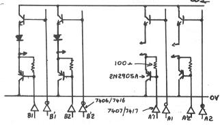
We have left NPN transistors for the top switches as the use of PNP's there gives us problems in their base drive circuits, but have replaced the bottom switches by PNP transistors.Note that the PNP's are drivem from buffers, not from inverters, to keep the input signals consistent with the earlier version of the drive circuit. The advantages of this circuit are;
