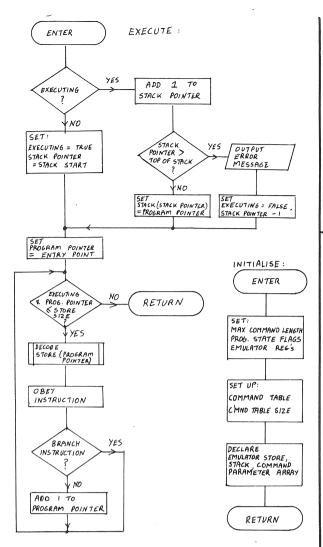
This flowchart may seem strange in places as it was drawn from a working BASIC PLUS program. As it is written, on starting, the program clears an area of memory (the emulator store, 256 l6 bit locations), sets a stack pointer to the start of the stack (25 l6 bit locations) and sets up the table of command (and instruction names). A line is then read with the presently required format;
